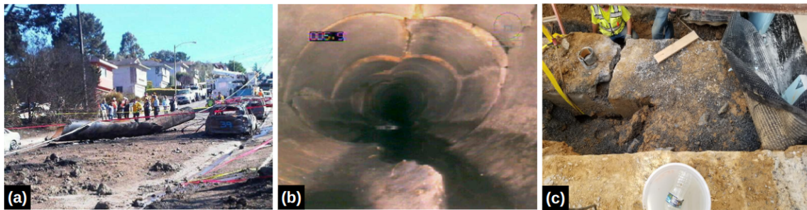
Figure 1.1: Examples of pipe failures. (a) Natural gas pipeline explosion in San Bruno, California, in 2010, resulting in eight fatalities [1]. (b) Severely deformed stormwater pipe still in service [2]. (c) Failure of a duct bank (a group of underground electrical conduits) [3].
