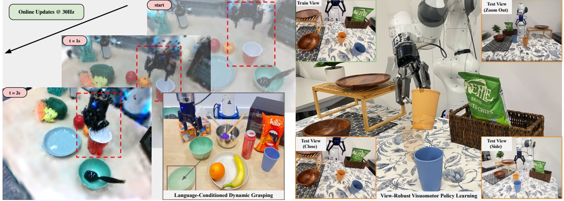
Figure 5.1: Object-centric Gaussian splatting. We propose a dynamic and semantic 3D representation based on Gaussian Splatting [47], which achieves an update rate of 30 Hz in response to robot and object movements. We show the reconstruction from different viewpoints of a grasping scene on the left. We apply this representation to obtain behavior cloning policies that are robust under various testing views even though only a single training view is available. We also apply our representation to enable zero-shot language-conditioned dynamic grasping.
