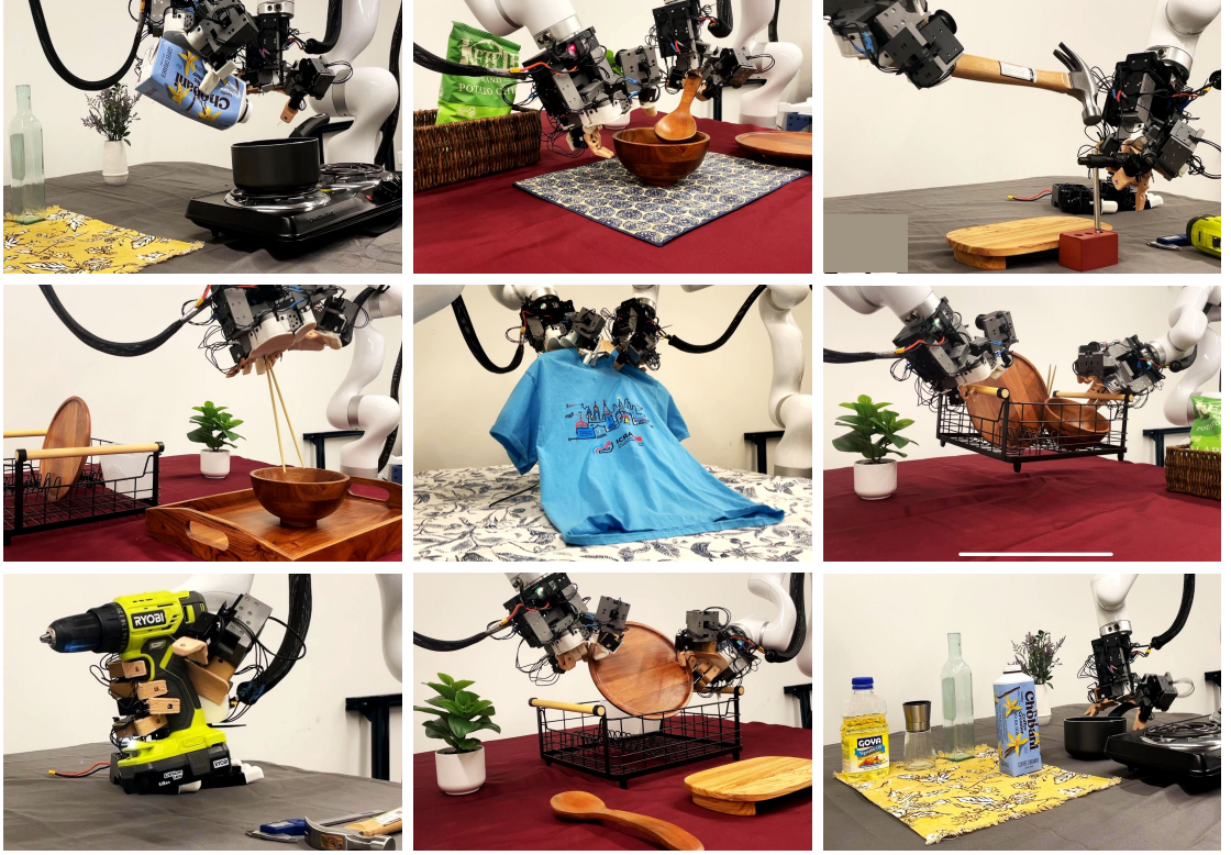
Figure 2.1: Bimanual Dexterity: BiDex can effortlessly teleoperate various complex tasks including pouring, scooping, hammering, chopstick picking, hanger picking, picking up basket, drilling, plate pickup and pot picking to train high-quality behavior cloning policies with over 50 degrees of freedom. Our teleoperation system and two LEAP hands [105] costs around $12k in total and is readily reproducible by academic labs.
