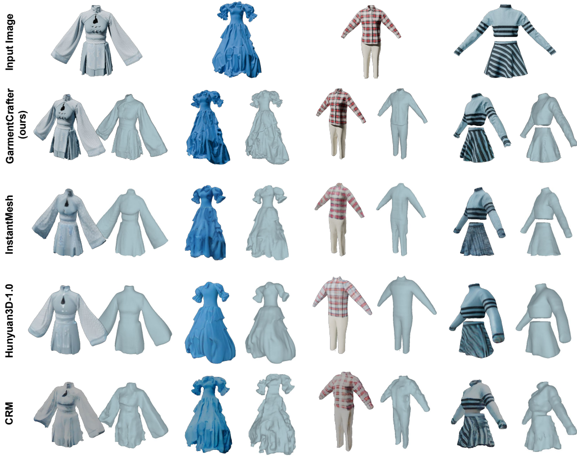
Figure 2.3: Qualitative comparison on single-view 3D garment reconstruction with state-of-the-art methods. Our method demonstrates better performance in handling complex texture patterns and geometric structures compared to InstantMesh [117], Hunyuan3D-1.0 [120], and Convolutional Reconstruction Model (CRM) [108].
