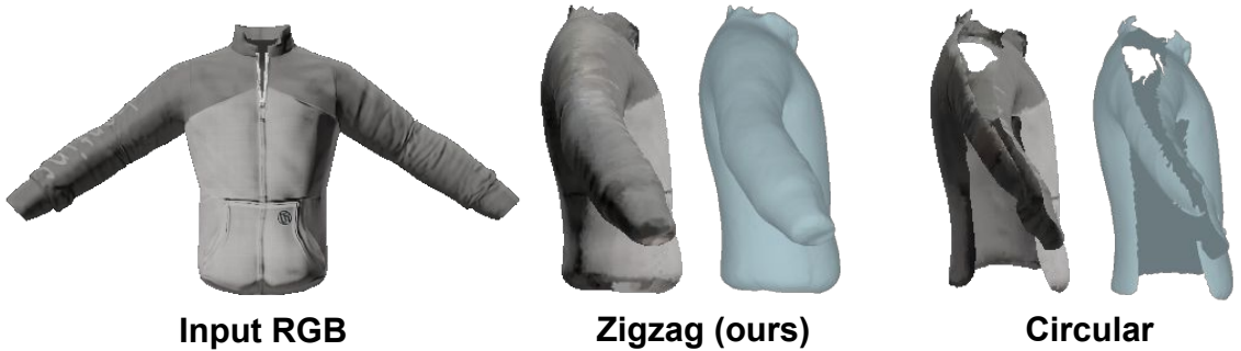
Figure 2.7: Camera trajectory selection for loop closure. Zigzag achieves better loop closure, while the circular trajectory struggles with side-view closure, leading to geometric conflicts and model failure. We argue that there are numerous ways to select camera trajectories, our proposed approach just offers an intuitive solution tailored for single-view garment reconstruction and editing.
