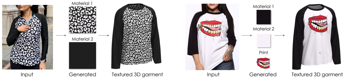
Figure 3.10: Multi-material textures transfer. Given a clothing image containing multiple texture patterns, materials, and prints, FabricDiffusion can transfer each distinct element to separate regions of the target 3D garment.
