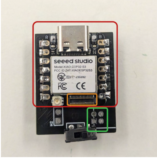
Figure 3.3: The front of the RESCUE Roller’s PCB contains an ESP32-S3 System on a Chip (Red), a connector for a camera breakout board (Orange) and additional through hole connections for I2C or SPI sensors (Green)
