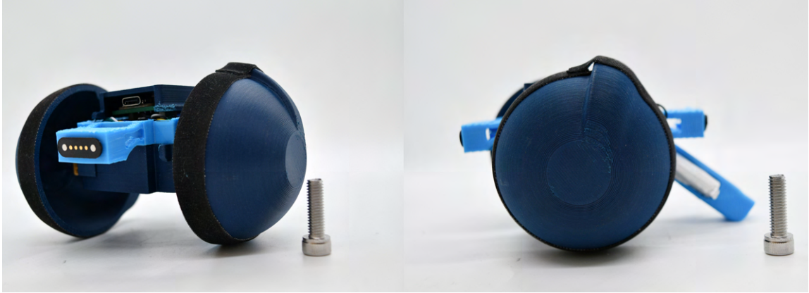
Figure 4.1: A fully assembled RESCUE roller from the front (left) and side (right). The tail monobody (light blue), is fabricated from thermal polyurethane (TPU) tail. The chassis and wheels (dark blue) are fabricated from polylactic acid (PLA). All parts were printed using a Bambu Labs X1. The systems battery and the magnetic connectors are featured in the tail. An M6 20mm bolt is included for scale.
