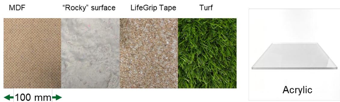
Figure A.9: Force testing materials. From left to right medium density fiberboard (MDF), our 3D printed “rocky” surface, LifeGrip tape on MDF, and turf.
