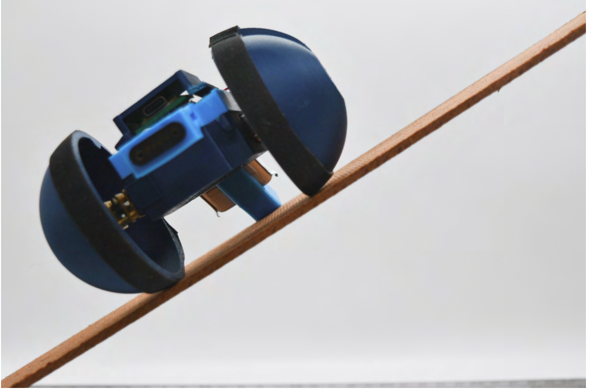
Figure 4.6: RESCUE roller on a 40 degree slope. With the adjustable wheel base we have a larger roll angle than in a fixed, small chassis case.
