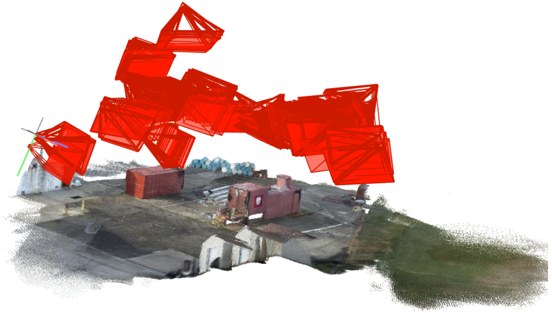
Figure 5.1: Qualitative results of VGGT [31] on the red container scene from our real-world dataset. VGGT identifies smoke as low-confidence points and enables effective removal of smoke through confidence-based filtering, resulting in a clean reconstruction of the underlying scene geometry.
