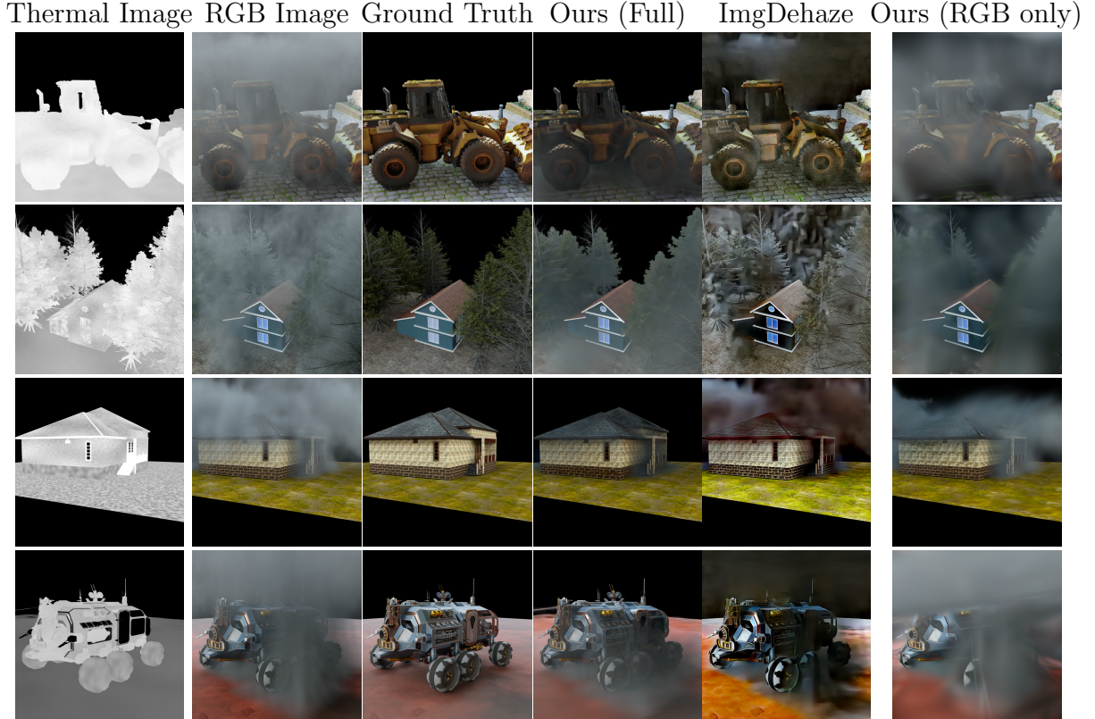
Figure 4.2: Qualitative results on the real dataset. From left to right: Thermal Image, RGB Image, Ground Truth, Ours (Full), ImgDehaze, and Ours (RGB only). Our method effectively removes smoke while maintaining the structural integrity and texture details of the scene.
