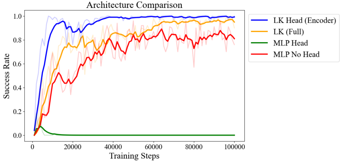
Figure 5.6: Success rate of different architectures over the training process. LK stands for "Learned Kinematics." Faint lines represent raw data, while solid lines show smoothed trends using an exponential moving average with \alpha = 0.3 .
