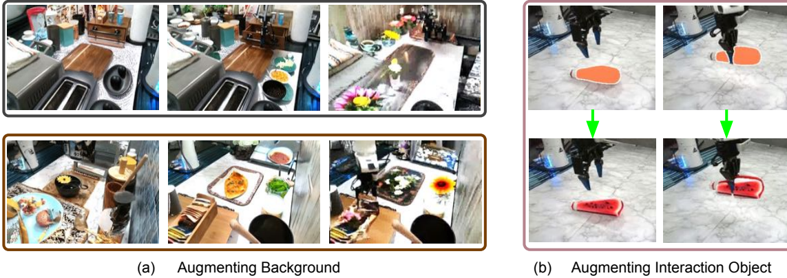
Figure 6.5: Illustration of the data augmentations used to rapidly multiply limited robot datasets with diverse semantic scene variations. (a) shows the scene around the robot and the interaction object changing. (b) shows the interaction object itself changing while preserving the rest of the scene.
