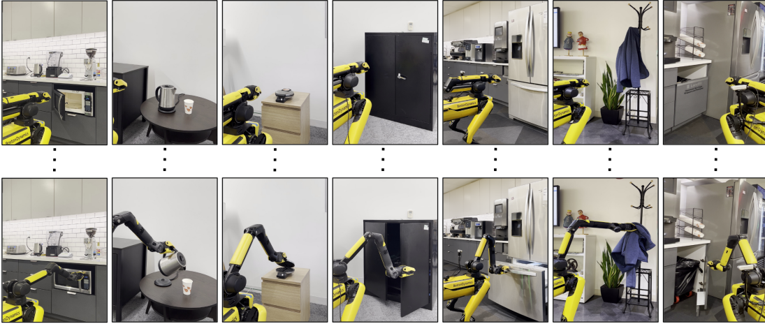
Figure 4.1: Glimpse of some of the diverse robot manipulation capabilities across physical office and kitchen scenes enabled by our framework. We learn to predict point tracks from web videos for learning interaction plans that can be used for inferring robot actions in unseen scenarios. This enables a common goal-conditioned policy to perform everyday tasks like closing microwaves, pulling out drawers, flipping open toasters, pouring from jars etc. Columns show first and last images of rollouts from our policy.
