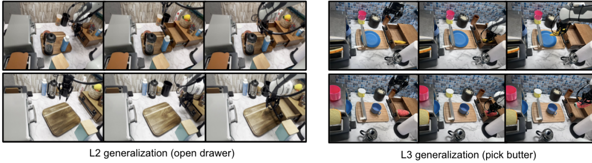
Figure 6.12: Qualitative results of rollouts for L2 and L3 levels of generalization, showing tasks open drawer and pick a slab of butter . For L2 we introduce different distractors in the scene, and change the background tiles. For L3, in addition to changes in L2 we introduce different task objects, for example by replacing a slab of butter with a piece of watermelon, or a banana.
