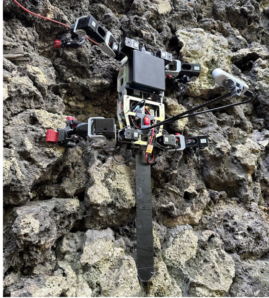
Figure 3.1: The LORIS robot uses passive microspine grippers and distributed inward gripping to ascend the side of a tufa stone bridge.
