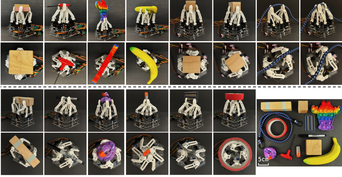
Figure 6.7: Grasping gallery with DELTAHANDS. We grasp (d) twelve daily objects with (a) a 9-actuator hand and (c) a 5-actuator hand. We also show (b) in-hand cube and rope repositioning.
