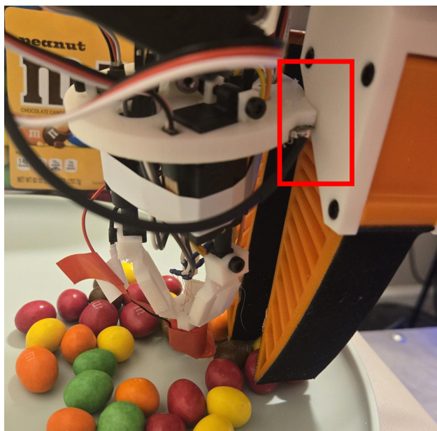
Figure 8.10: Contact between the Delta Finger platform and the two Fin Ray fingers when the Fin Ray fingers are fairly close prevent the third finger from being able to go between the fingers and help with a M&M singulation task.
