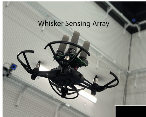
Figure 6.1: A Flow Shadowing 2 x 2 grid of whiskers on a micro quadroter in flight. Scale bar represents 100 mm
