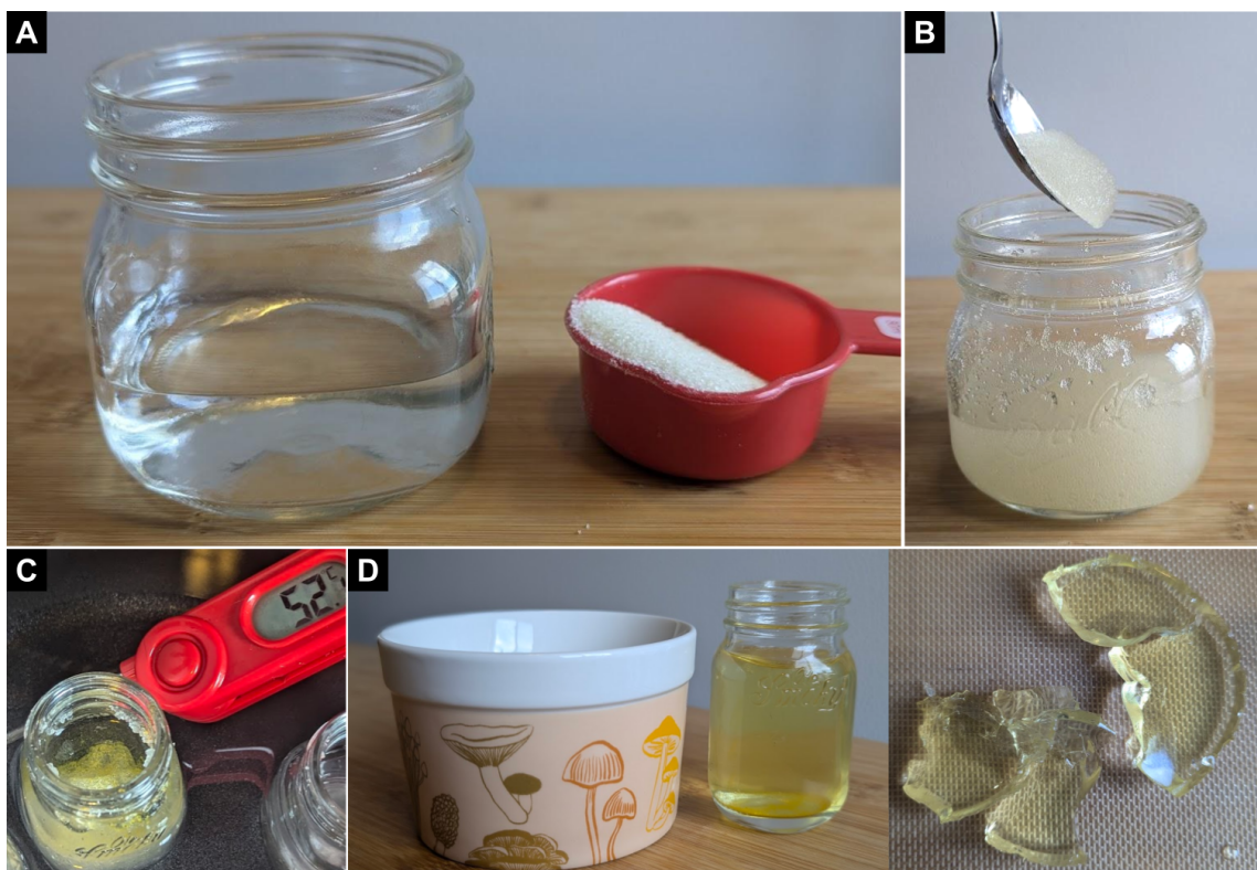
FIGURE 4.2: A) Tap water and pristine gelatin powder. B) Gelatin powder hydrated by slow addition to water (blooming, resulting in a paste). C) Melting gelatin in a stove-top water bath with a commercial probe thermometer for temperature monitoring. D) Ramekin and molten gelatin sol-phase for casting. E) Fresh, swollen, pristine hydrogel without additives
