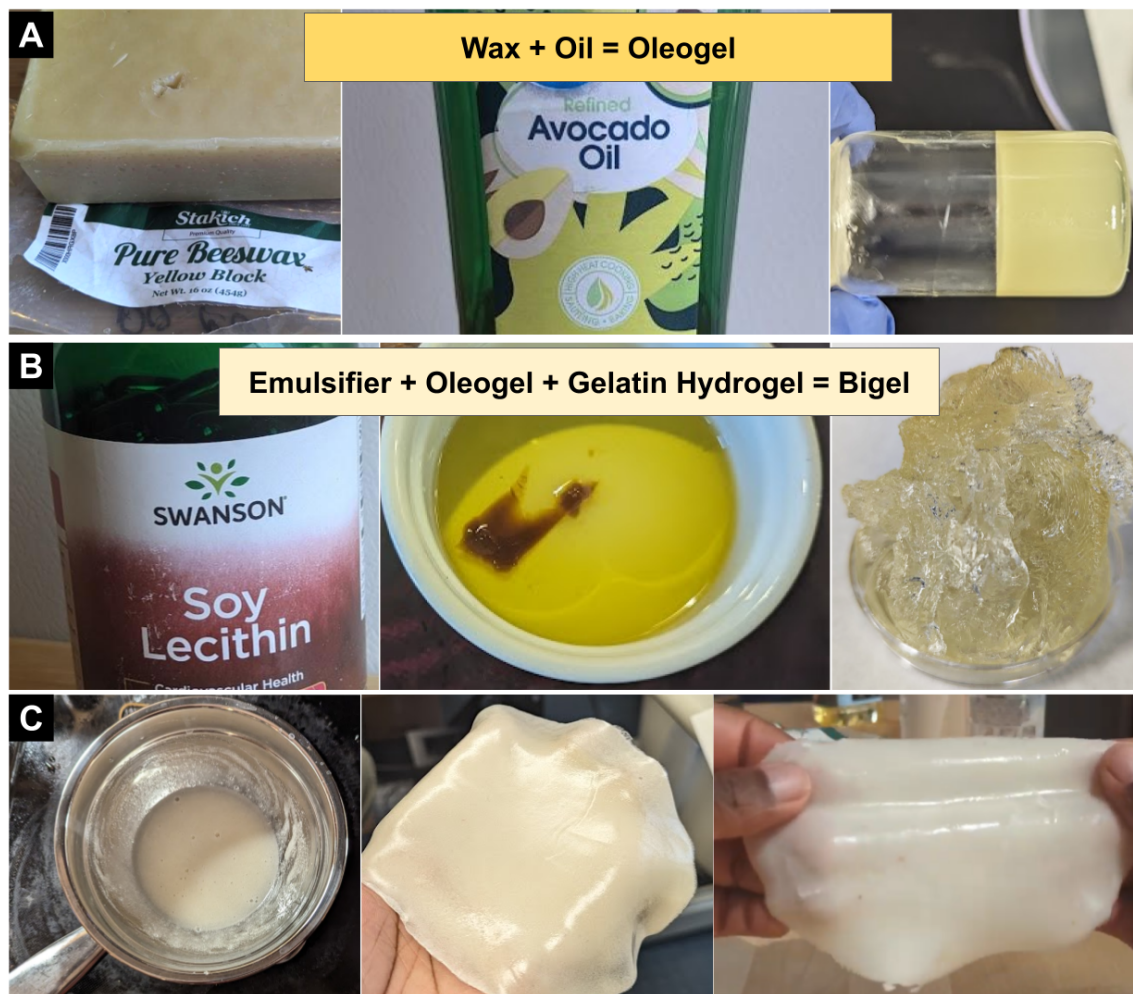
FIGURE D.2: A) Oleogel and its ingredients. B) Emulsifier, molten oleogel, and coagulated gelatin hydrogel. C) Combined bigel, flexible and slightly stretchable.
