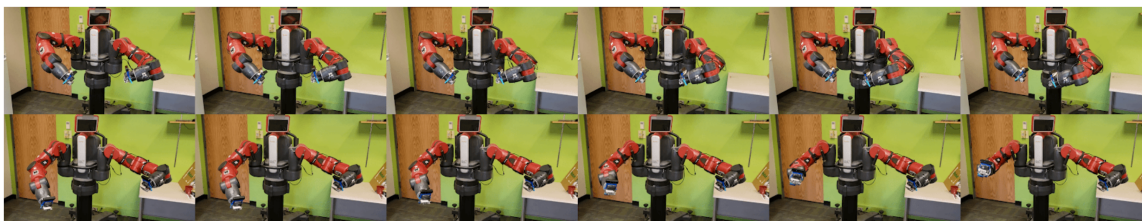
Figure 3.4: Depiction of execution of the learned primitives on real world Baxter robot. Each row is a single primitive, while columns show progress of the primitive over time. Row 1 depicts a left handed reaching primitive, while row 2 shows a right handed returning primitive. More visualizations provided in supplementary material, and videos are provided in the webpage.
