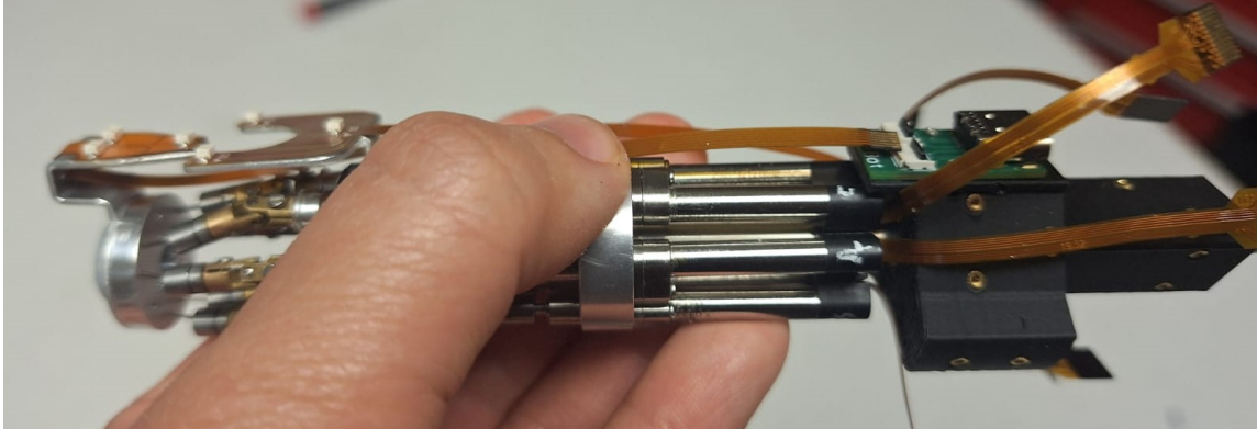
Figure 5.12: PCB and ASAP Mounts connected to the manipulator.
