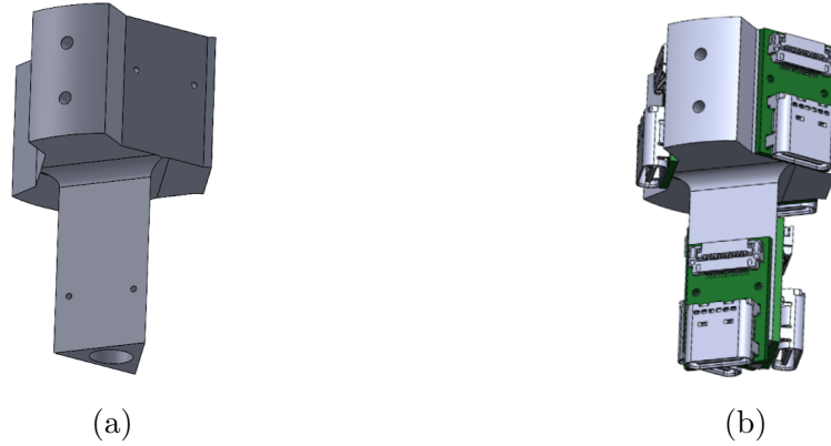
Figure 5.11: PCB mount CAD drawings: a) PCB mount without PCBs, b) PCB mount with PCBs.
