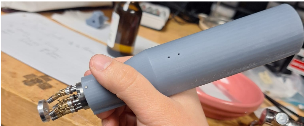
Figure 5.15: The printed handle attached to the manipulator.
