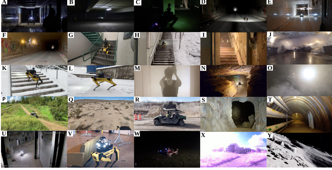
Figure 3.3: The SubT-MRS datasets were collected across diverse seasons, capturing environments with perceptual challenges such as poor illumination, darkness, and water puddles, where visual sensors falter. They also include geometrically complex areas like long featureless corridors and steep multi-floor structures, challenging LiDAR systems with potential drift. Moreover, these datasets cover conditions with airborne obscitants like dust, fog, snow, and smoke in tough environments, including caves, deserts, long tunnels, and off-road areas.
