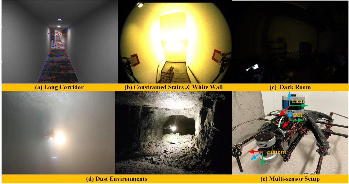
Figure 5.1: (a-d) shows the challenging environments where we collect datasets. (e) shows our multi-sensor setup.
