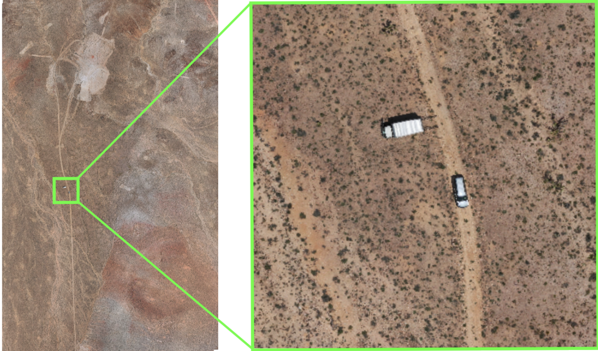
Figure 1.7: Ortho image from a field dataset spanning an area of 900x700 meters, showcasing its high spatial resolution of 3 cm/pixel
