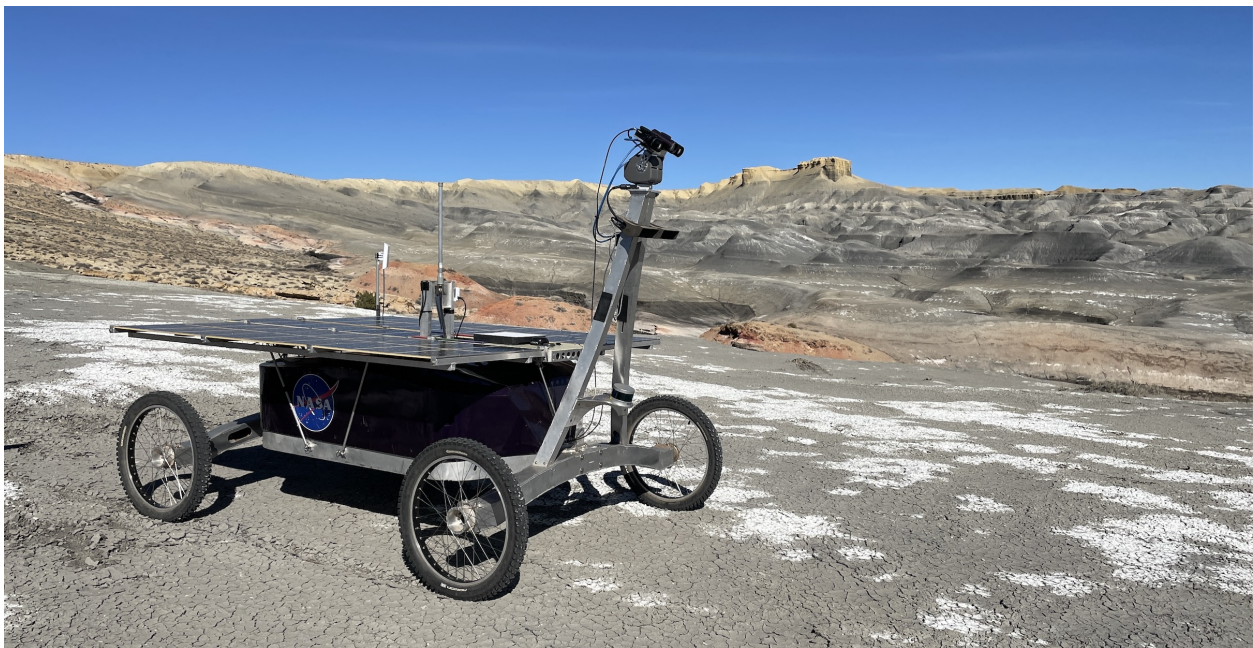
Figure 1.5: Zoë is a solar powered field robot with an onboard spectrometer (ASD FieldSpec Pro) and can measure wavelengths in visible, NIR and SWIR bands ranging up to 3000 nano meters. It uses a one-degree fore-optic mounted on a pan/tilt to measure surrounding terrain
