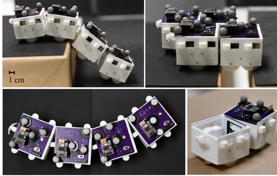
Figure 4.1: Top: Robots can form a flexible chain and go down a step (left) or a rigid structure that crosses a gap between two equal-height platforms (right). Bottom left: Four robots forming an articulated chain. Bottom right: One robot inserts its anchor inside the opening of another one (circuitry removed for visual purposes).
