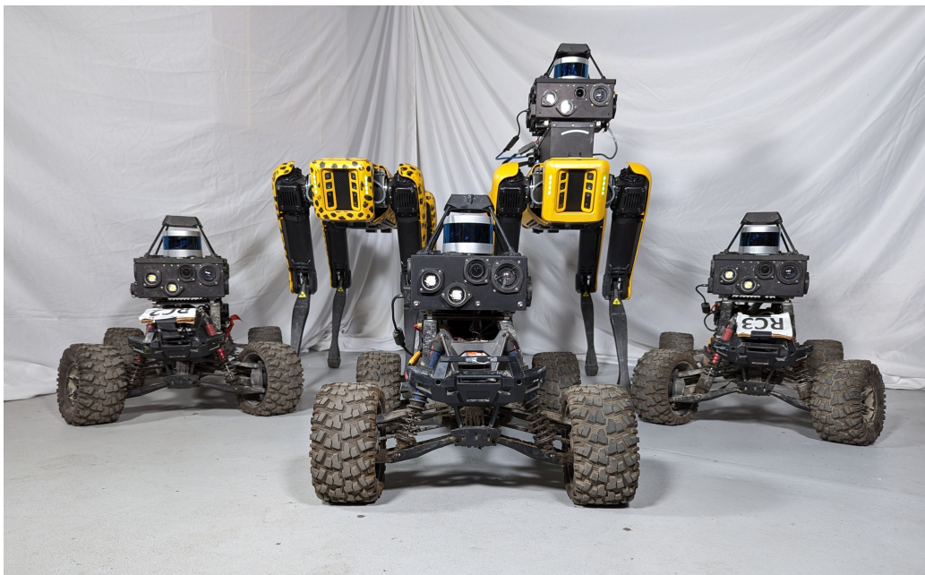
Figure 1.5: Various robots with LiDAR sensors attached; Credit: Matt Lab
