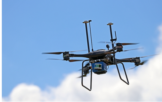
Figure 1.2: A drone flying with LiDAR sensor attached on top; Credit: Near Earth Autonomy
