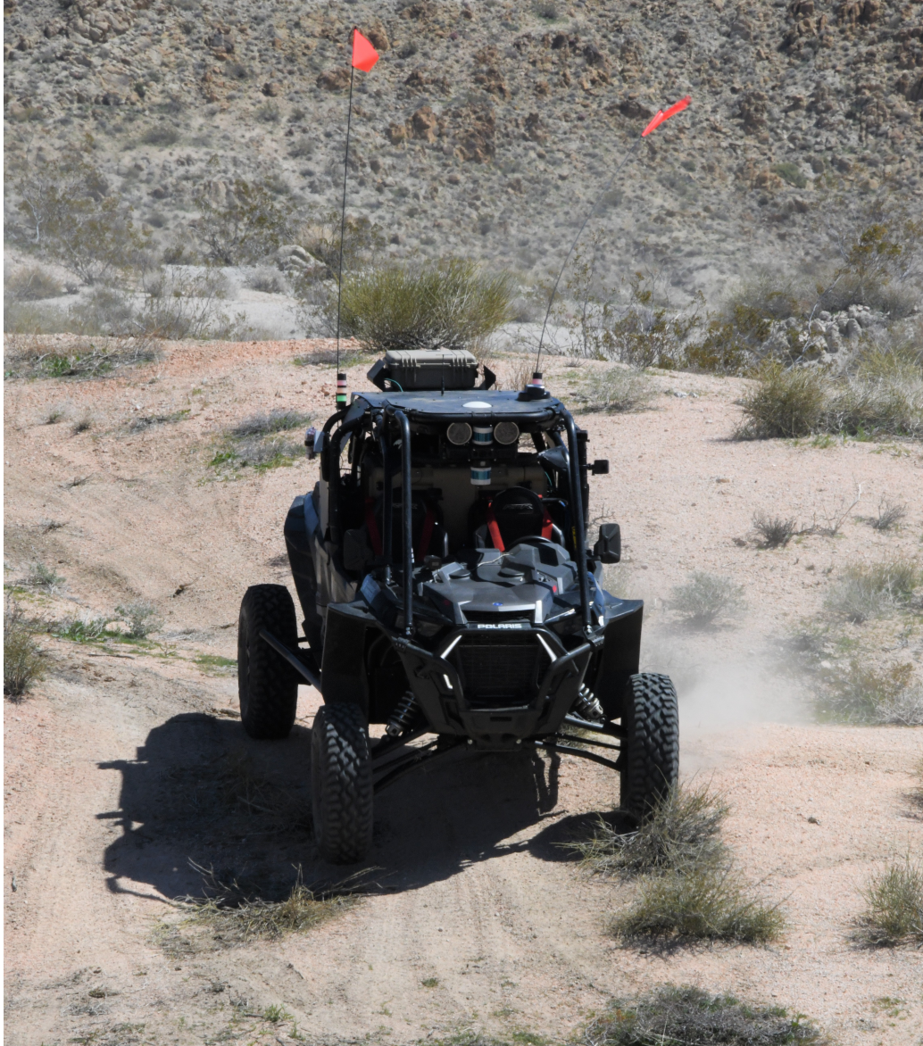
Figure 1.4: A vehicle driving with LiDAR sensors attached; Credit: DARPA RACER Website
