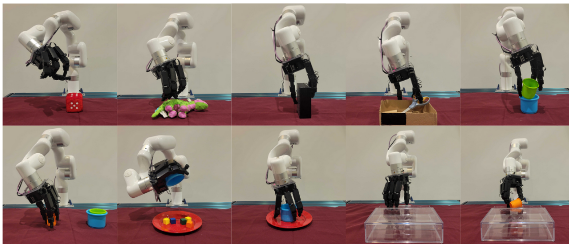
Figure 4.7: Ten different teleoperation tasks. Top row, left to right: Pickup Dice Toy, Pickup Dinosaur Doll, Box Rotation, Scissor Pickup, Cup Stack. Bottom row, left to right: two cup stacking, pouring cubes onto plate, cup into plate, open drawer and open drawer and pickup cup. Please see videos at https://robotic-telekinesis.github.io/ .
