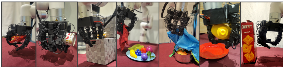
Figure 5.5: Tasks used in experiments. From left to right: pick, rotate, open, cover, uncover, place and push. See https://video-dex.github.io for videos of these tasks.
