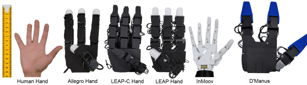
Figure 2.1: Relative size of popular robot hands to scale. Left to right , adult human hand, Allegro Hand [5], LEAP-C Hand, LEAP Hand, Inmoov [16], D’Manus [51]. LEAP Hand is similar in size to Allegro and \sim 30\% larger than a human hand. D’Manus is considerably larger than the rest. Because of the tendon-driven nature, Inmoov is the smallest robotic hand. The hands are accurate to scale.
