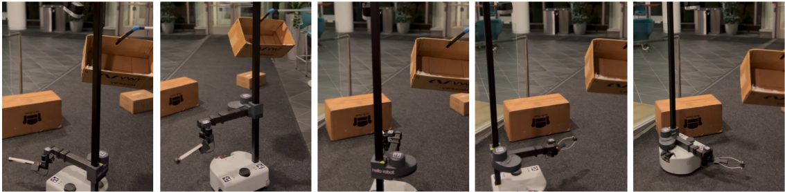
(c) The robot adapts its plan on-the-fly to obstacles by turning around once the camera sees it.
