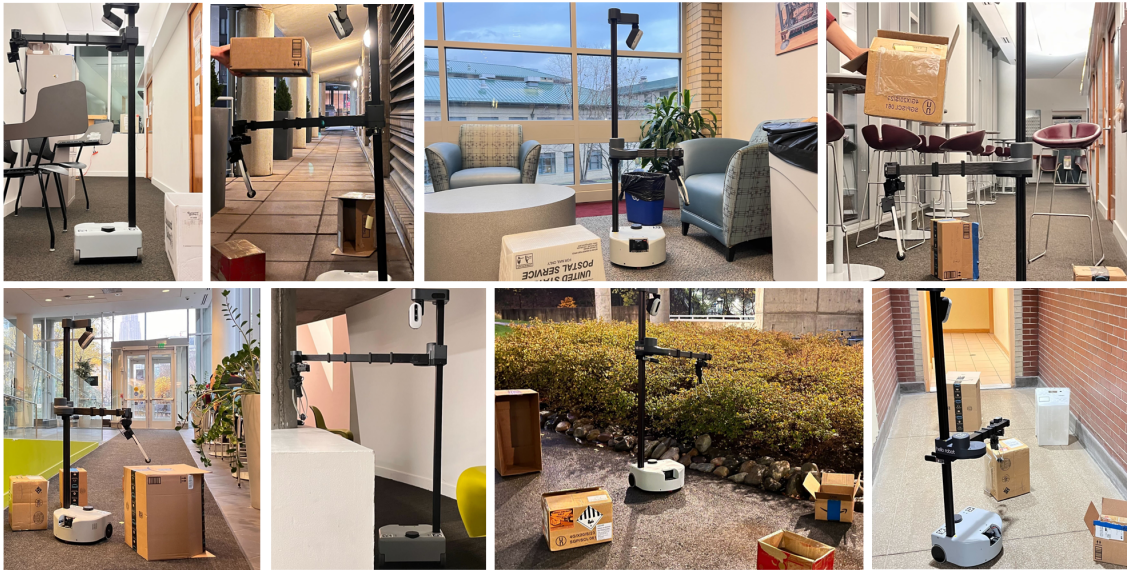
Figure 1.2: Learning to SPIN: Our robot learns to Simultaneously Perceive, Interact, and Navigate around cluttered unstructured environments in a whole-body fashion. The robot has an actuated camera with a limited field of view that it must control to get information about its environment. The motion and perception problem are tightly coupled since what the robot knows about the environment influences how it can move and vice versa. We show results in a large variety of scenarios both indoors and outdoors with different obstacles like boxes and furniture. Our robot can pick up different objects like cups, and utensils. Video demos at https://spin-robot.github.io
