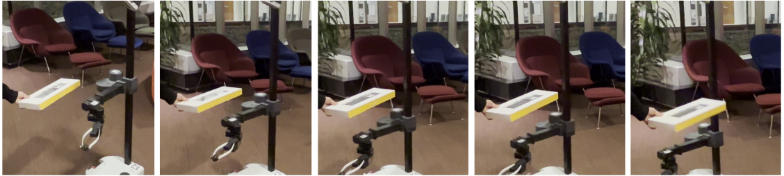
(b) If there is an overhanging obstacle, the robot lowers its arm to avoid it instead of turning around, thereby displaying agile whole-body coordination.
