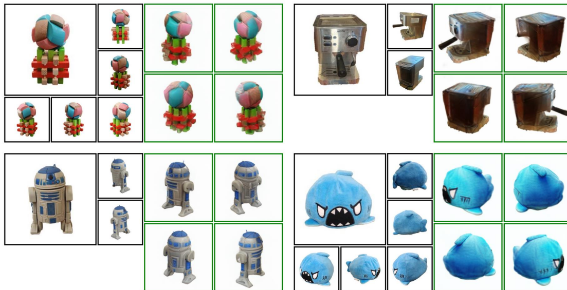
Figure 4.5: 3D from self-captured images. Given 3-6 self-captured input images for a generic object (left), we show 4 novel viewpoints of the 3D asset recovered via UpFusion † (3D) (right).
