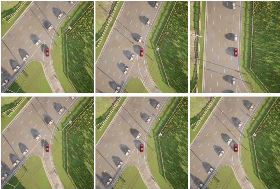
Figure 4.3: Qualitative example of proactive merging with closed-loop planning. The top row is from our proposed closed-loop planner and the bottom row is from the open-loop variant of our planner. Frames are in sequential order from left to right. The closed-loop planner merges proactively in front of other cars, causing the car behind to yield to the ego-agent. The open-loop planner does not predict that the ego will affect the behavior of other cars, so it does not attempt to merge.
