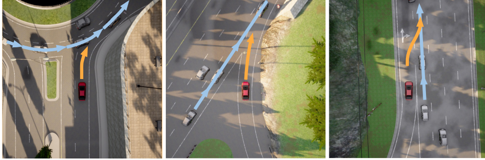
Figure 4.2: Merge scenario visualization. The red car is the ego-vehicle, the orange arrow indicates the desired merging behavior, and the blue arrows indicate the flow of traffic in the target lane.
