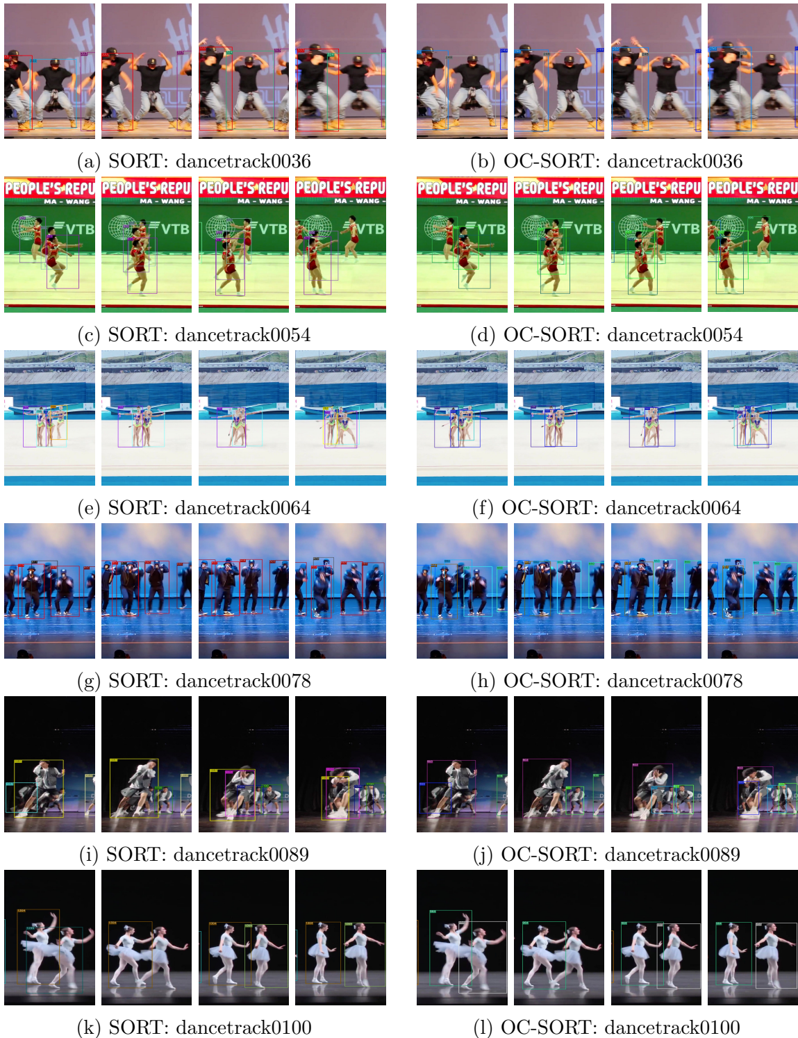
Figure 4.1: More samples where SORT suffers from the fragmentation and ID switch of tracks from occlusion or non-linear motion but OC-SORT survives. We selected samples from diverse scenes. Best viewed in color and zoomed in.
