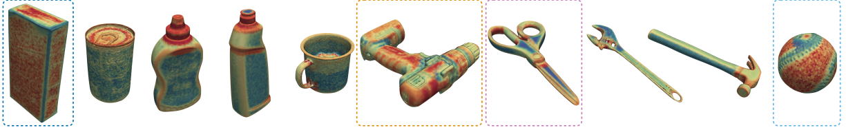
Figure 4.3: Tactile codebook per object visualized as a spectral colorspace map using t-SNE [VH08]. Each codebook comprises of 50k densely sampled poses with their corresponding 256-dimensional tactile code. Similar hues denote sensor poses that elicit similar tactile codes. We can clearly delineate local geometric features: edges (sugar_box), ridges (power_drill), corners (scissors), and complex texture (baseball).
