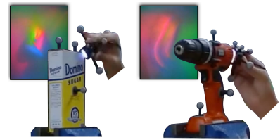
Figure 4.6: Real-world sliding trials in the YCB-Slide dataset. Inset is an example tactile image from the interactions, capturing the local geometry of the object.
