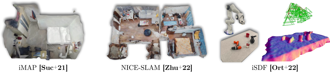
Figure 5.2: Online learning has been applied in RGB-D SLAM for indoor and tabletop scenes. iSDF [Ort+22] has been shown to reconstruct room-scale and tabletop scenes from posed depth images. iMAP [Suc+21] and NICE-SLAM [Zhu+22] also perform camera tracking via the differentiable renderer, in conjunction with SDF optimization.
