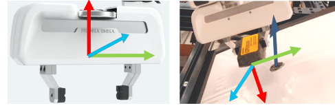
Figure 3.3: Left : Palm keypoint with an arbitrary frame. Right : Tool keypoint with EE frame and surface normal (black arrow) for black mark on the board. The other in-plane axes for the black mark are much more arbitrary.
