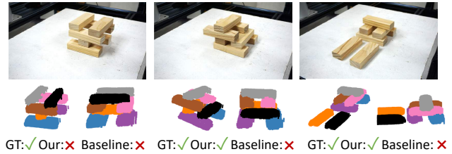
Figure 5.5: Left : Example scenes for block unstacking task. Right : Test set examples for block unstacking task. The black block shows the block to be removed. Baseline here refers to visual baseline.
