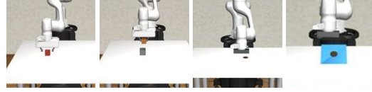
Figure 3.5: Robosuite [269] tasks used to evaluate the efficiency of using our structured skill representation approach. From left to right – Lift, Stack, Wipe, Wipe with slanted board.
