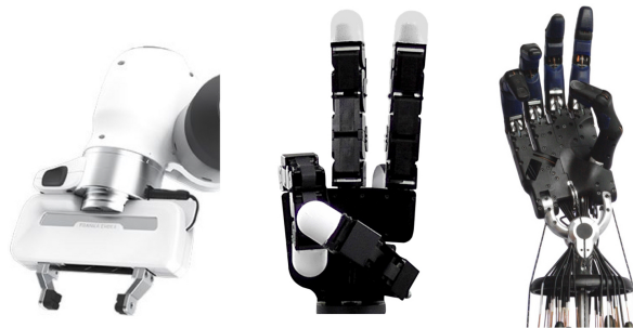
Figure 1.1: Popular state-of-the-art (rigid) manipulators: (Left) two-finger gripper attached to a Franka robot arm [1] (Middle) Allegro dexterous hand [2] and (Right) ShadowHand [3].
