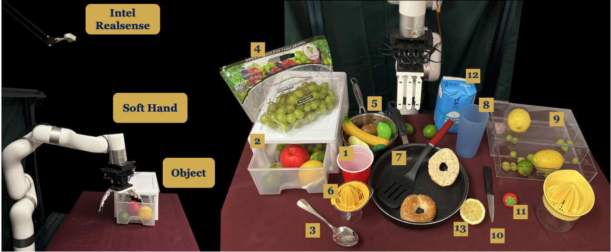
Figure 6.3: Left: Workspace Setup. We place an Intel RealSense camera above the robot to maintain an egocentric viewpoint, consistent with the affordance model’s training data. Right: Thirteen objects used in our experiments.
