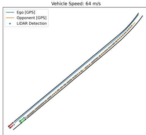
Figure 5.10: Sequence 2 from Attacking at the 125\text{mph} speed. Each sequence is 7 seconds long. During the pass, the vehicle reached a peak speed of almost 150\text{mph} . By the time the vehicles enter the turn, our vehicle has completed the pass and begins to drop back to the round speed. During the entire sequence, the stack is able to detect and track the other agent, providing the planner a reliable belief of where the other agent is, allowing for a safe pass, even at such high speeds.
