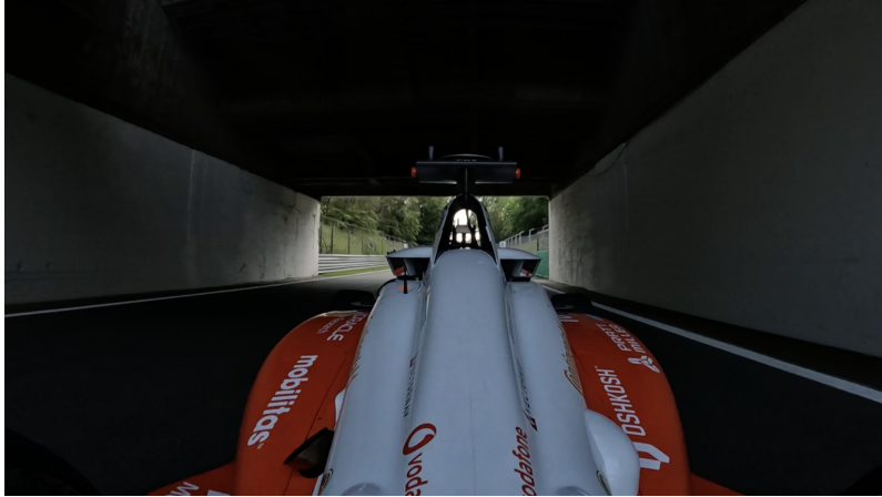
Figure 4.2: One section of the modern Monza track runs under the old track. GPS reception is completely obstructed while in the tunnel. Additionally, the track leading up to the tunnel has dense tree coverage, which creates multi-path interference and obstructs reception. The result is a challenging environment for GPS-based localization.
