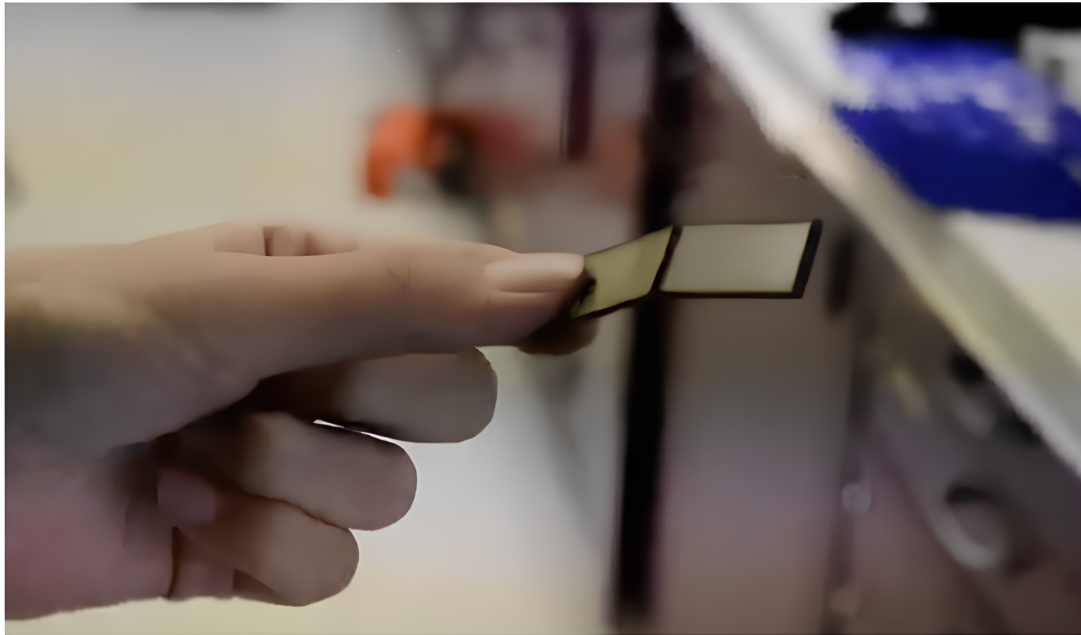
Figure 2.4: 5-layer laminated piece with the FR4 as the rigid layers and exposed bioplastic layer in the middle as flexure joint.
