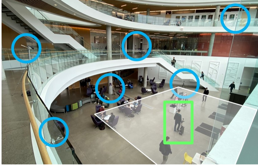
Figure 8.2: Hardware setup for the TBD Pedestrian Dataset. Blue circles indicate positions of RGB cameras. The green box shows our suitcase robot pushed through the scene. The white area is where trajectory labels are collected. The data collection area is much larger for Set 2.
