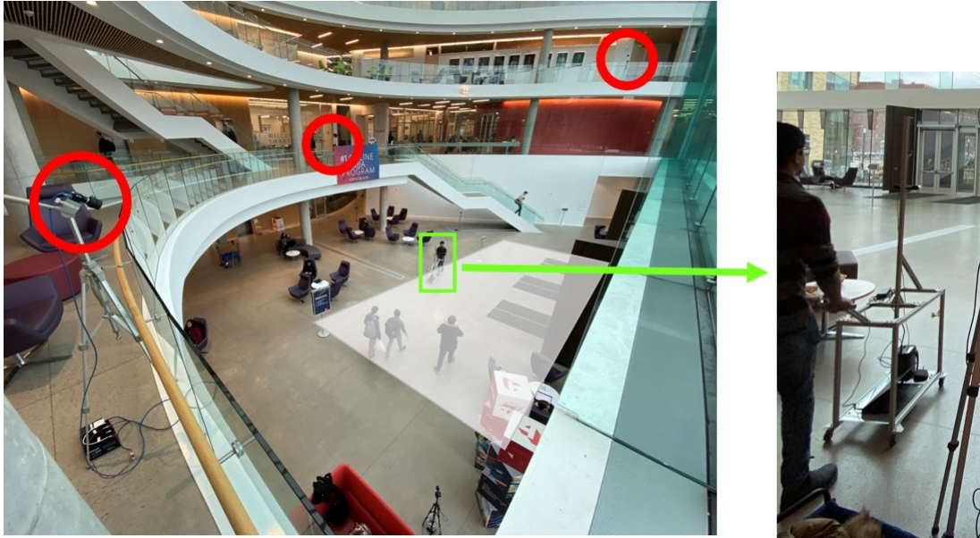
Figure 7.2: Hardware setup for the TBD Pedestrian Dataset. Red circles indicate positions of RGB cameras. The green box shows our mobile cart with a 360° camera and stereo camera which imitate a mobile robot sensor suite. The cart is manually pushed by a researcher during recording. The white area is where trajectory labels are collected.
