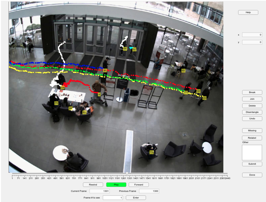
Figure 8.3: App interface for the human verification process. It contains a media player and various options to fix tracking errors automatically and manually.
