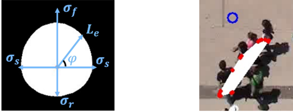
Figure 3.2: Left: A sample individual social space. Right: A sample group space from simulated laser scans. Note that the lower-right pedestrian is occluded from the ”robot” (blue circle) and is not included in the group.
