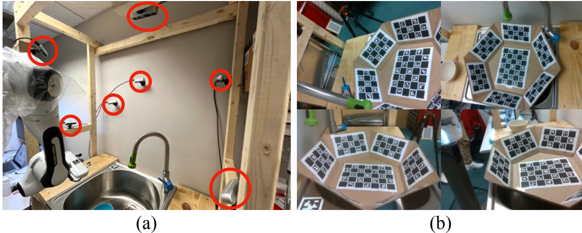
Figure 2.3: Camera Setup and Calibration. Eight RealSense D435 depth cameras, seven of them shown in (a), strategically positioned around the sink area, capturing different angles and perspectives for comprehensive depth perception. Calibration board is shown in (b), used for determining the camera intrinsics and extrinsics.
