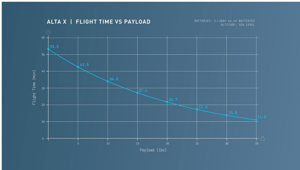
Figure 3.4: Estimated flight times for the Freefly Alta-X [3]
