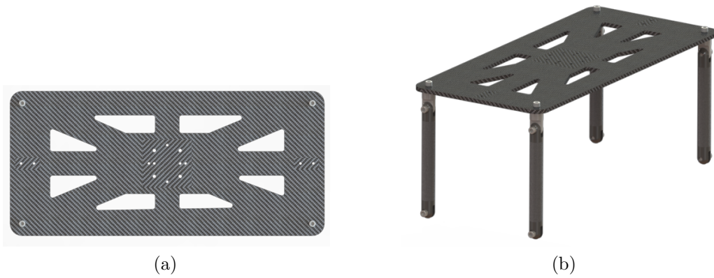
Figure 3.24: Mounting plate for Freefly Alta X: (a) top view, (b) isometric view
