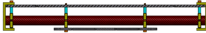
Figure 3.25: Front view of the main structure of the sensing payload. Color code: aluminum (yellow), nylon (cyan), carbon fiber (red/black), steel (orange)
