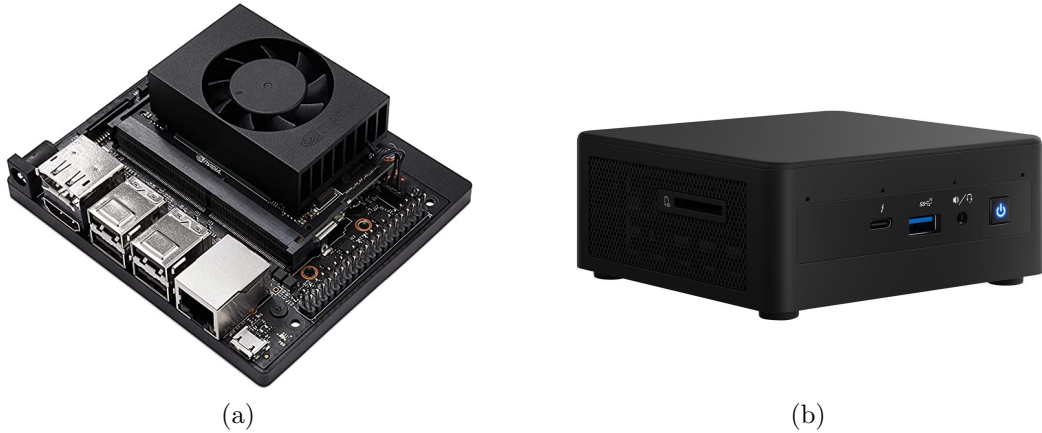
Figure 3.11: Onboard computers: (a) NVIDIA Jetson Xavier NX Development Kit, (b) Intel NUC 11
