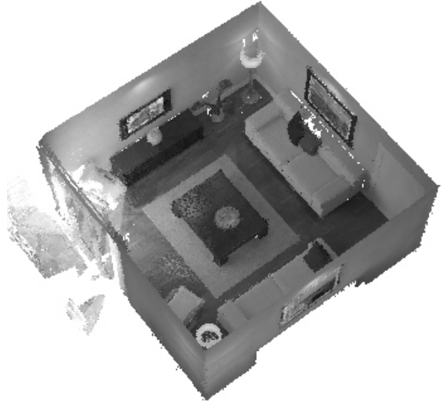
Fig. 1: A reconstructed point cloud using spatial and intensity information inferred from the compact multimodal point cloud model created using the proposed approach. The representation leverages a formulation that has been demonstrated to be amenable for higher level robot autonomy objectives like exploration in complex, unstructured 3D environments. A video is available at: https://youtu.be/VgPEEcbUAnY .
