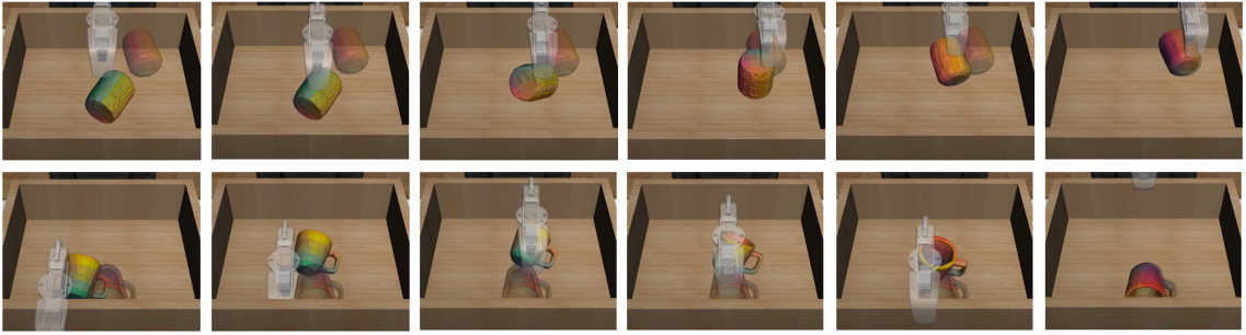
Figure 5.5: Qualitative results for the object pose alignment task. HACMan shows complex non-prehensile behaviors that move the object to the goal pose (shown as the transparent object).
