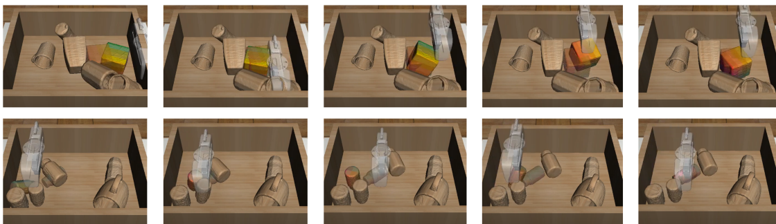
Figure D.9: Qualitative results for object pose alignment tasks in cluttered environments. HACMan shows complex non-prehensile behaviors that move objects to goal poses (shown as the transparent objects). The scene objects are colored in brown to distinguish from the target object to be manipulated to the goal pose.
