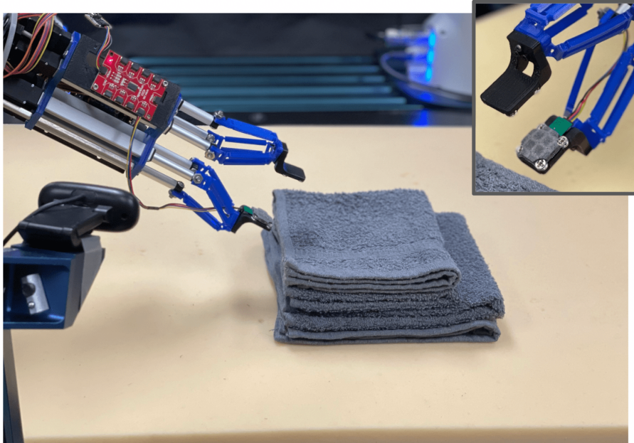
Figure 5.1: We present a tactile-based cloth manipulation system. The robot utilizes a ReSkin [8] sensor attached to the lower one of its two fingertips, which is visualized in more detail in the upper right inset. We train a classifier to distinguish among grasping different numbers of cloth layers from tactile feedback (no images are provided as input). The robot then uses this classifier at test time to determine suitable grasping points for obtaining a desired number of cloth layers.
