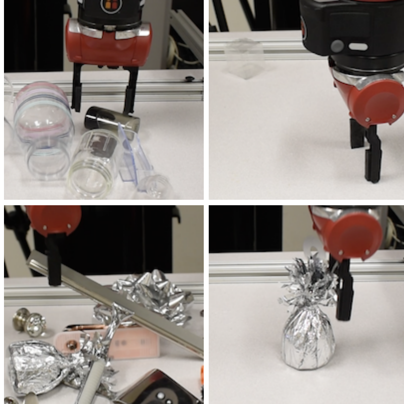
Figure 2.7: Examples of failure cases. (top left) Grasp does not account for transparent part of sharpener. (top right) Gripper fails to detect transparent plastic cube and grasps at table. (bottom left) Mass distribution of squeegee causes grasp to fail. (bottom right) Foil on top of balloon weight appears graspable but the gripper passes through.
