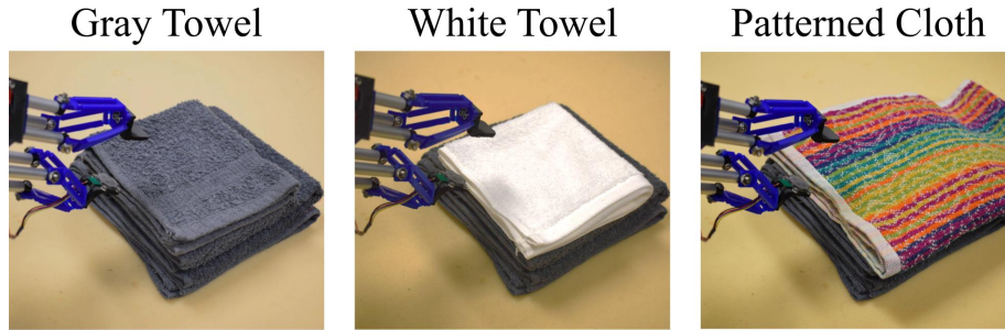
Figure 5.6: The cloths we use for experiments. We use the gray towel (left) for training, and test on all 3 cloths for evaluation. The white towel and patterned cloth test generalizing to novel cloths. The cloths have thicknesses between 3-5 mm and variation in surface texture and stiffness.
