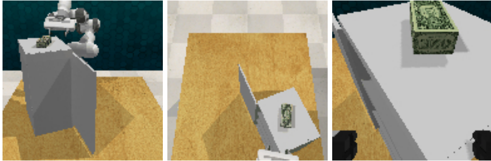
Figure 6.2: Visualization of the three views used in this set of tasks: front, top, and wrist-mounted.
