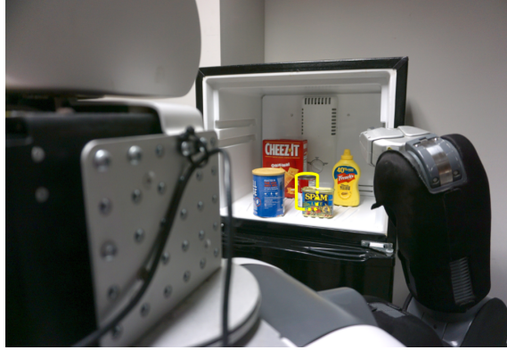
Figure 4.8: Real-world setup for pick-and-place MAMO experiments with a PR2. The tomato soup can (yellow outline) is the object-of-interest.
