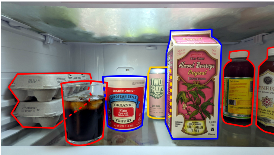
Figure 6.1: The goal is to retrieve the beer can (yellow outline). The yogurt and almond beverage are movable objects (blue outlines). All other objects in the scene are immovable obstacles (red outline).
