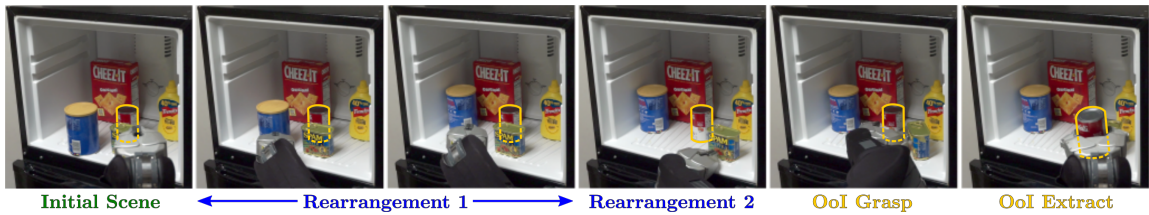
Figure 4.7: A MAMO solution generated by M4M . The tomato soup can (yellow outline) is the OoI, all other objects are movable.
