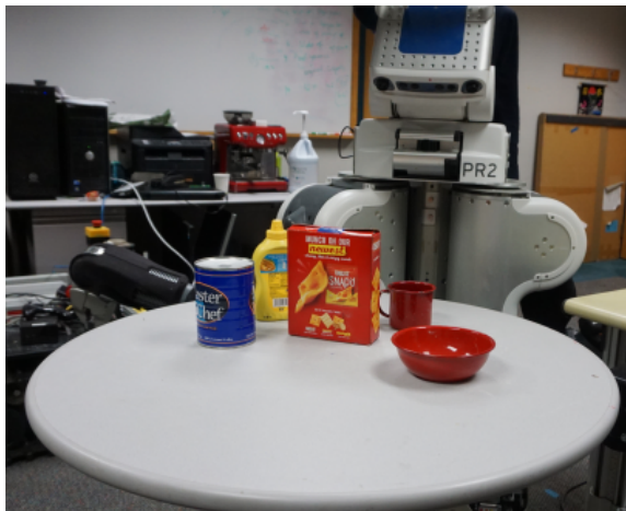
Figure 3.6: Experimental setup for a PR2 robot in front of a tabletop workspace for MAMO.
