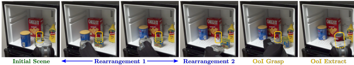
Figure 1.3: A PR2 robot executing a solution trajectory found by M4M for a real-world MAMO problem.
