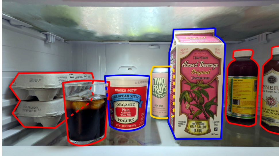
Figure 1.1: The goal is to retrieve the beer can (yellow outline). The yogurt and almond beverage are movable objects (blue outlines). All other objects in the scene are immovable obstacles (red outline).
