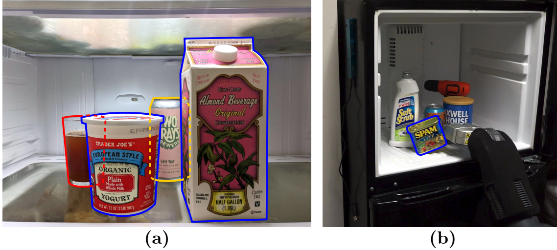
Figure 4.1: (a) An example MAMO problem to retrieve the beer can (yellow outline). Access is blocked by the movable box of milk and tub of yogurt (blue outlines). In order to retrieve the can, they must be rearranged out of the way without toppling them, and without anything making contact with the glass of juice (red outline). (b) A complex non-prehensile action that tilts the movable potted meat can (blue outline) to rearrange it.
