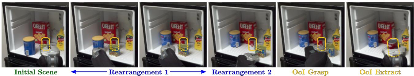
Fig. 7. A MAMO solution generated by M4M. The tomato soup can (yellow outline) is the OoI, all other objects are movable.
