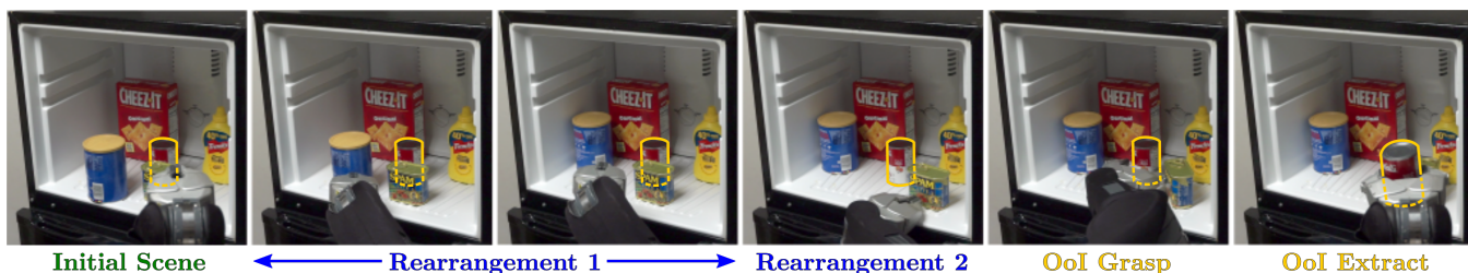
Figure 7: A MAMO solution generated by M4M. The tomato soup can (yellow outline) is the OoI, all other objects are movable.
