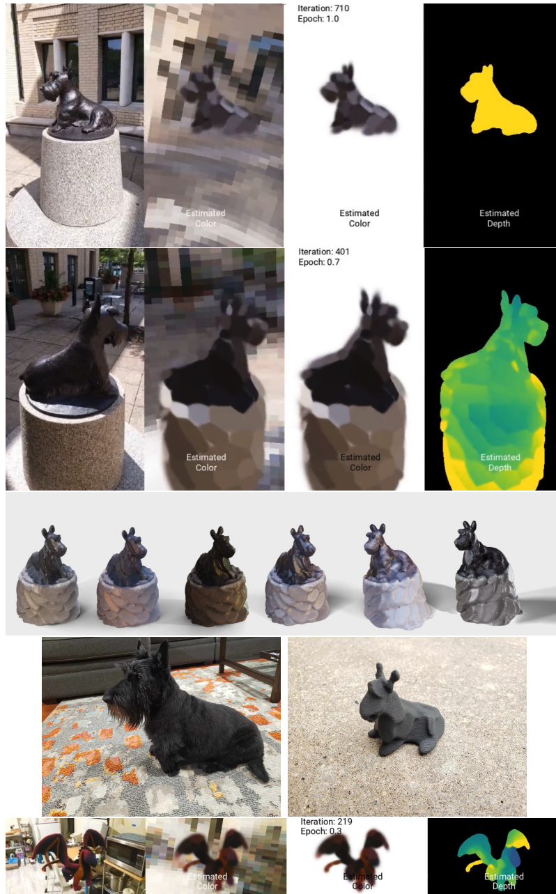
Figure 3.11: Reconstruction of Scottish Terrier Statue on the Carnegie Mellon Campus. Performed by running SAM [Kir+23] on the first frame and propagating with XMem [CS22], before performing the optimization described in this section. Different reconstructions with different masks are possible, as is relighting the reconstructed meshes in Blender. Charlie, my actual Scottish Terrier, is shown for reference. As is a printed 3D model of 32 Gaussian reconstruction of the object. And a dragon (crocheted by K. Shih) reconstruction to represent CMU SCS.
