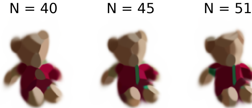
Figure 3.10: Re-parameterized 3D Gaussians to minimize apparent loss. N is the number of mixtures used. The appearance of the tie and the sleeve in green can be seen with added Gaussians.
