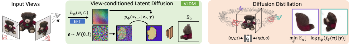
Figure 4.1: Overview of SparseFusion. SparseFusion comprises of two core components: a view-conditioned latent diffusion model (VLDM) and a diffusion distillation process that optimizes an Instant NGP [20, 39]. We use VLDM to model p(\mathbf{x}|\boldsymbol{\pi}, C) .
