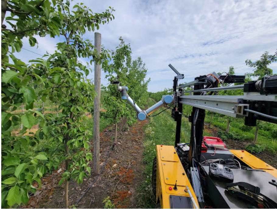
Figure 6.2: In-hand flash stereo camera [93] attached to a 7 DoF robotic arm [94].
