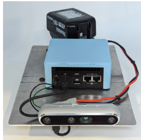
Figure 4.2: A sensor payload with RealSense D455 RGBD sensor and an Intel NUC compute
