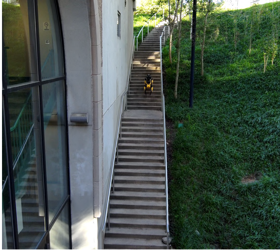
Figure 4.6: The Spot robot traversing a long staircase as a test of the staircase system and its merging capabilities in real-time
