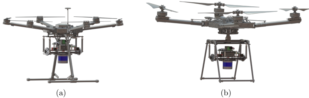
Figure 3.2: Aerial platforms with sensing payload mounted: (a) DJI M600 Pro (b) Freely Alta X
