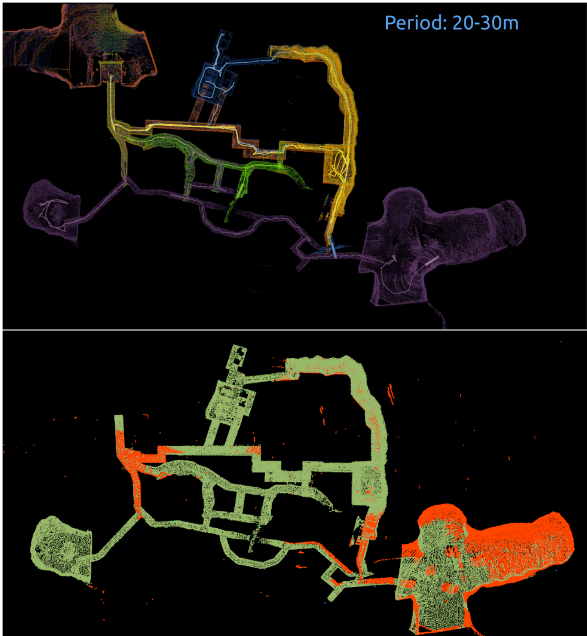
Figure 1.1: Top: Complete map generated by Team Explorer after 30 minutes in the Final Event. Multiple colors represent contributions from different robots. At this stage, Team Explorer had reached 26 out of 28 map sectors, as defined by DARPA. Bottom: Final complete map colored by the deviation metric. Green are inlier points, within 1 meter of ground truth. Orange are outlier points.
