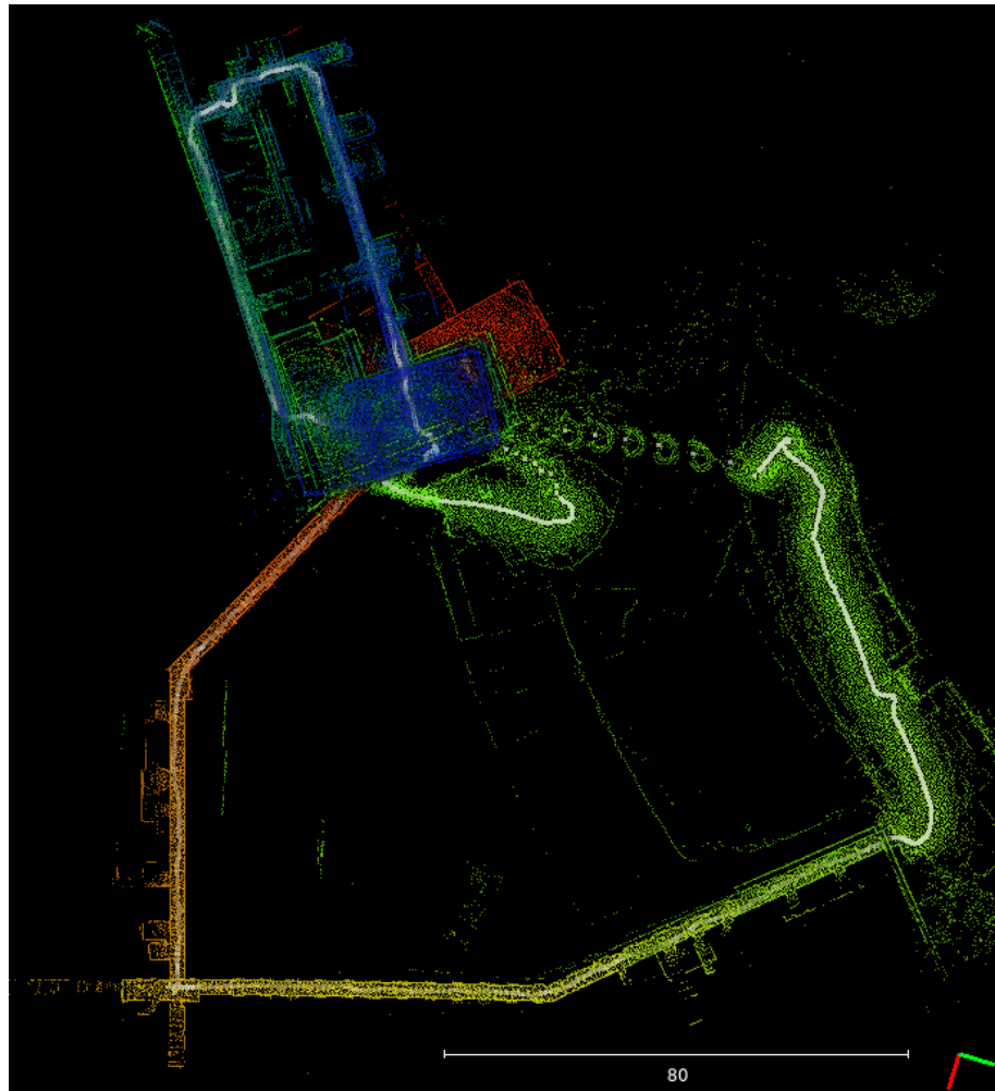
Figure 5.6: Indoor-Outdoor With Failure dataset. Pointcloud is colored by point acquisition time. Robot trajectory is shown in white. Notice the section where the trajectory becomes discontinuous, which leads to drift and failure in mapping.
