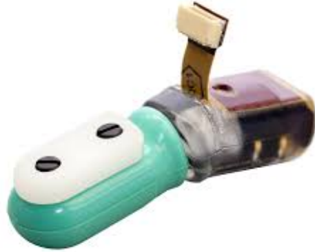
Figure 2.5: Image taken from company website. This image depicts the bioTac sensor.
