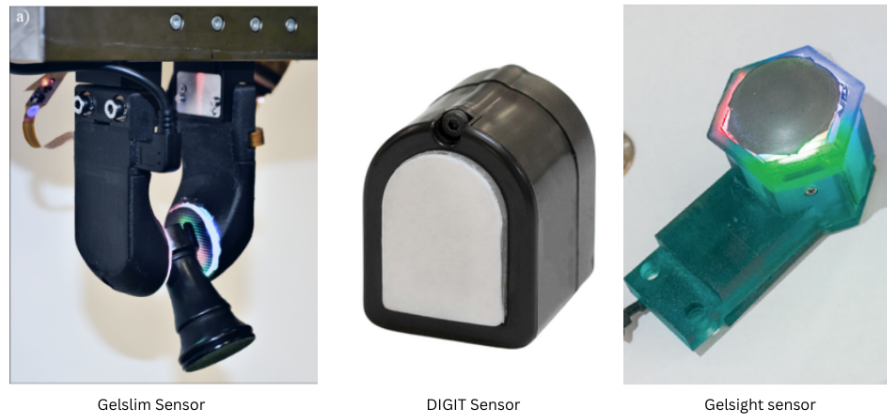
Figure 2.1: Different Optical Gel Based sensors. Gelslim, Digit and Gelsight from left to right.
