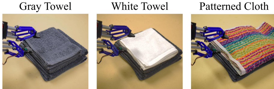
Figure 3.6: The cloths we use for experiments. We use the gray towel (left) for training, and test on all 3 cloths for evaluation. The white towel and patterned cloth test generalizing to novel cloths. The cloths have thicknesses between 3-5 mm and variation in surface texture and stiffness.
