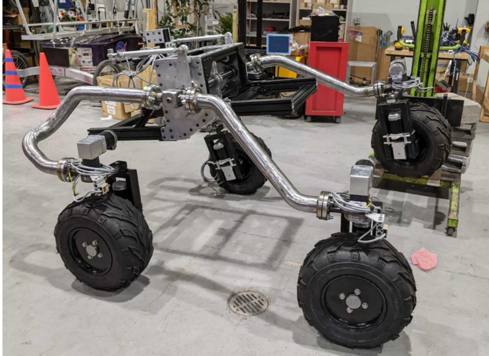
Figure 3.1: The effect of the rocker mechanism in averaging the chassis angle
