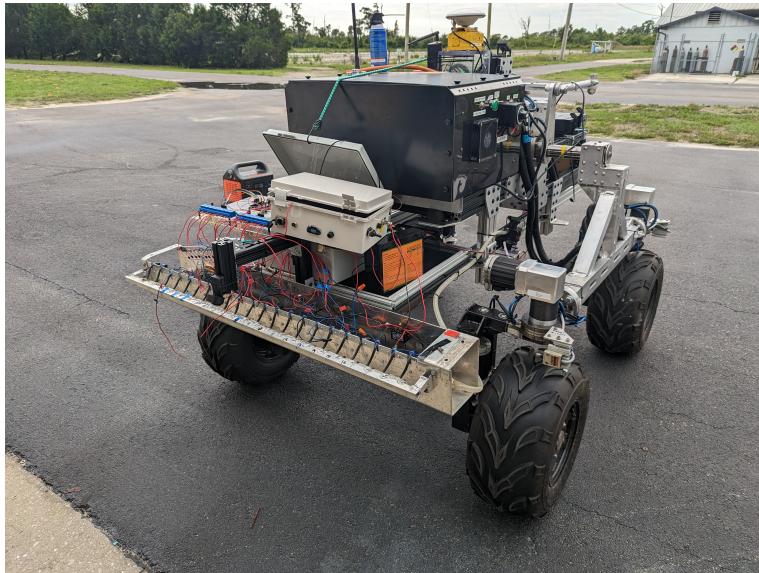
Figure A.1: Spraying unit mounted on robot
