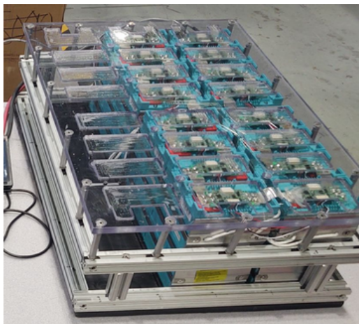
Figure 3.10: Large battery bank
