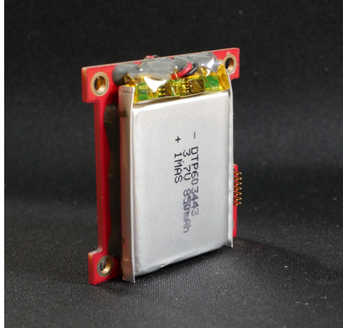
Figure 2.15: LiPo cells installed on a middle-batteryboard (second cell not visible)
