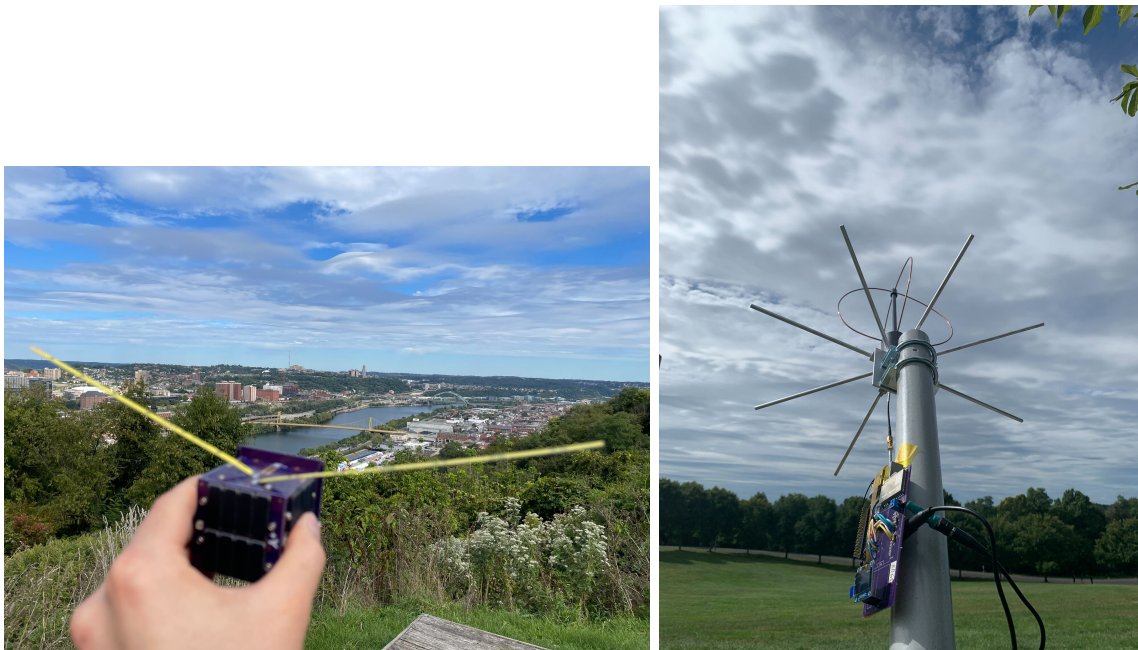
Figure 3.15: Photographs from a long-distance satellite communication test. PyCubed-Mini (left), ground station and antenna (right)
