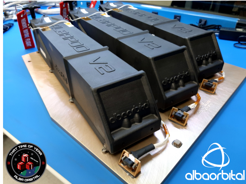
Figure 3.1: AlbaPod V2 PocketQube deployment pods, constructed out of Windform XT 2.0 composite. credit: Alba Orbital
