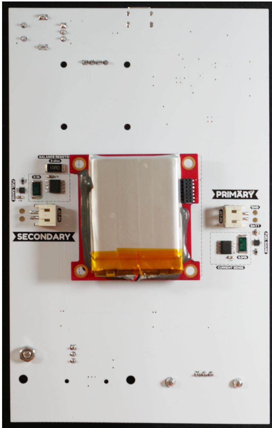
Figure 3.11: Power Tester Board: Back View - The batteries are mounted to the bottom of the tester boards to shield them from direct light. The boards are manufactured with a white solder mask to prevent overheating under the grow lights.
