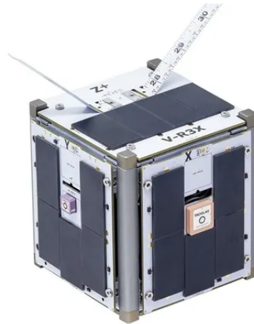
Figure 1.1: V-R3x: A 1U CubeSat nano-satellite developed by the Robotic Exploration Lab (RExLab)
