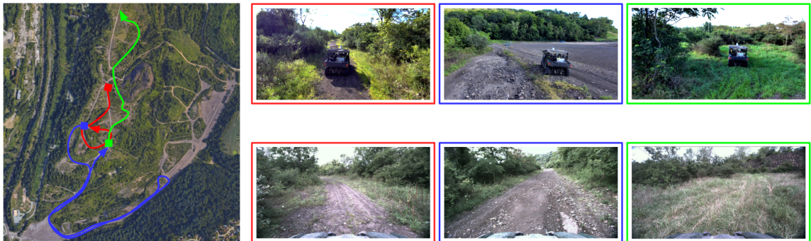
Figure 3.8: Overview of large-scale navigation experiments. The leftmost figure shows a satellite view of the three courses: red, blue, and green. The top row shows sample aerial views of the courses, while the bottom row shows sample first-person robot images. The color of the rectangle around the picture denotes the course.
