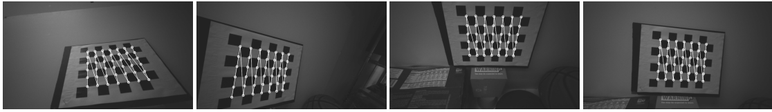
Figure 4.3: Sample checkerboard captures with detected corners. 100+ checkerboard poses are used to span both cameras' field of view at different depths and orientations to accurately calibrate for the camera parameters.
