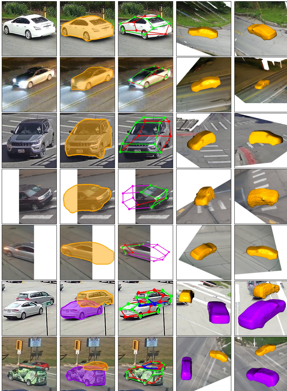
Figure 4.13: We show additional qualitative results on multiple sequences of the WALT dataset. The input image ( col 1 ) to the pipeline produces amodal segmentation mask ( col 2 ) and keypoint locations ( col 3 ). in ( col 4 and 5 ), We visualize the 3D reconstruction from multiple views
