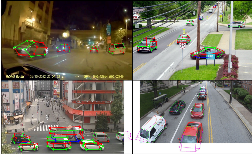
Figure 4.5: Sample images from our proposed Occlusion Category Classification (OCC) Dataset. The dataset contains a wide range of appearance variations including day and night and various traffic scenarios, accompanied by human-annotated keypoint locations and occlusion type (color-coded).
