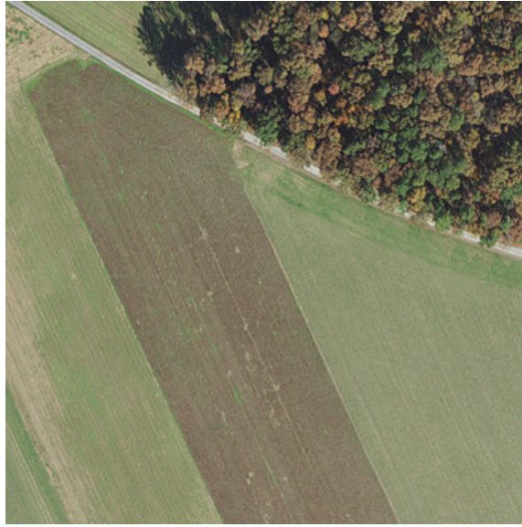
Figure 4.2: An example NAIP image crop at a resolution of 0.6 meters per pixel. Land cover classes are generally easy to interpret, but small details are lost.
